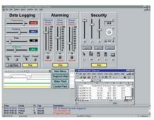
Lookout *Direct* provides you with an alarm set that most other packages offer, plus more. It triggers alarms with an event or any combination of events you specify. Alarms can be as simple or as complex as needed. The alarming is so versatile that you can group your alarms in any manner, turn off any nuisance alarms, prioritize them, and acknowledge alarms and events from anywhere in the network.
