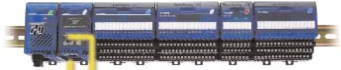
Ethernet Base Controller's (TIH-EBC) on-board serial port provides a link to label printer/appliator
