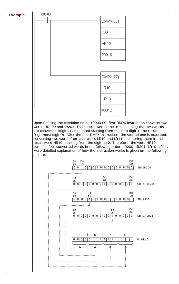
Presuming that binary value is the one from locations IR200, IR201, LR10 and LR11, as in example, the result of conversion in the result word HR10 would be "5B7D".
