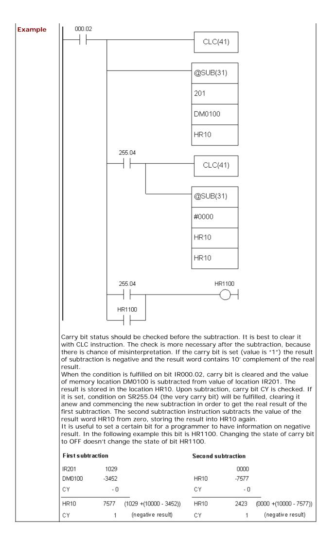
Character "@" ahead of SUB(31) represents the differencial form of the instruction, or simply put, this instruction will not execute non-stop while the condition is fulfilled. Only changing the condition from OFF to ON executes the instruction. This means that the second subtraction instruction won't take place immediately after the first one. Before executing the second instruction, it is necessary that bit IR000.02 changed state from OFF to ON at least once.
